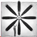
The world's largest and highest capacity propeller is a Curtiss-Wright Turboelectric. Designed for use with an extremely high-powered turboprop engine, this 17-foot diameter, eight-bladed light metal one now being tested by the Air Force, employs the steel reaction principle developed by Curtiss-Wright in 1941.
